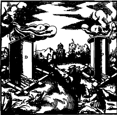
Figure 1a. Type 1 ventilating device for directing a blowing wind down a mine shaft. At the top of the crossed vanes a round disc forces the winds F downwards into the shaft (Source: De Re Metallica).
