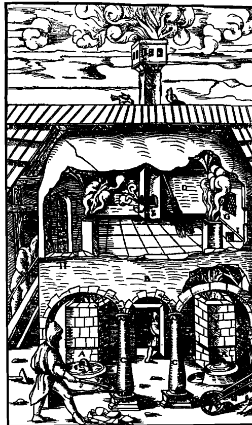
Figure 2. Dust chamber (D) for collecting particles from the gases before they escape through the opening (E) in the chimney (F) (Source: De Re Metallica).
