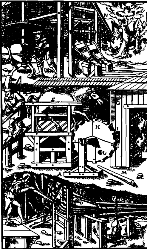
Figure 1c. Type 3 ventilating device in which bellows are used to move the air (Source: De Re Metallica).
