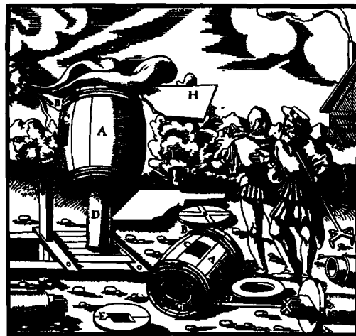
Figure 1b. Type 2 ventilating device with a swivelling collector of fresh air to collect the breezes and send them down the ventilator pipe D (Source: De Re Metallica).
